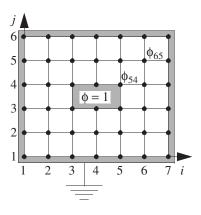
4) For the mesh given in the figure, number all nodes according to the Cuthill-McKee algorithm. Repeat the procedure twice treating nodes A and B as root nodes. In both cases determine the half-bandwith of the matrix.
